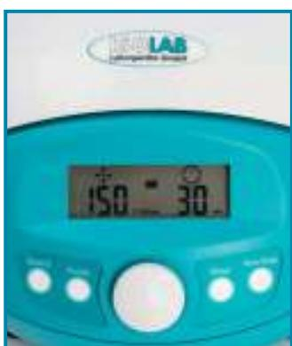
User friendly large LCD display enables easy setting and reading of the functional parameters. Both RPM and RCF can be set and displayed.
